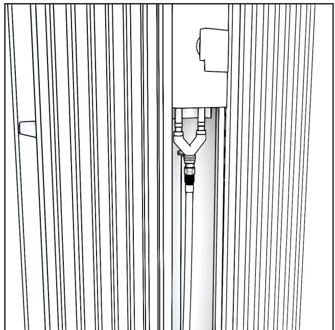
2. Thread the garden hose through the hole at the bottom of the outdoor shower and into the wall, then connect it to the shower.
