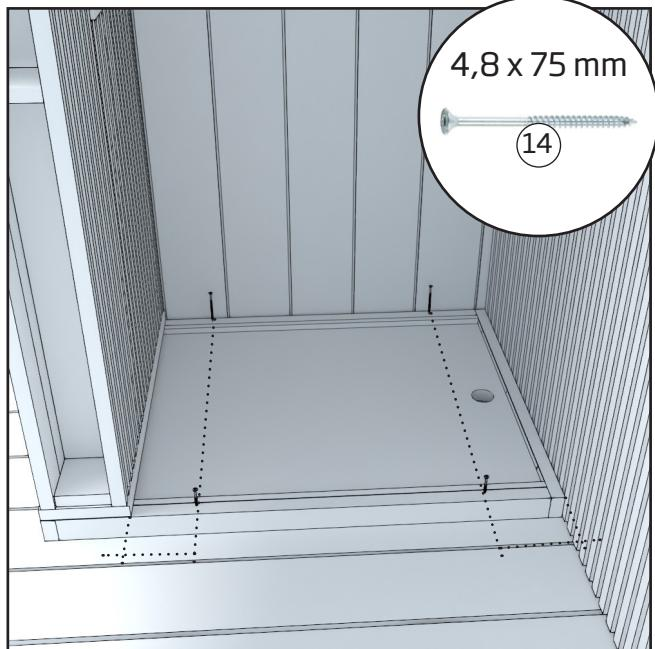
Lift off the grate and screw the base onto the terrace deck. Put the base grate back in place.
