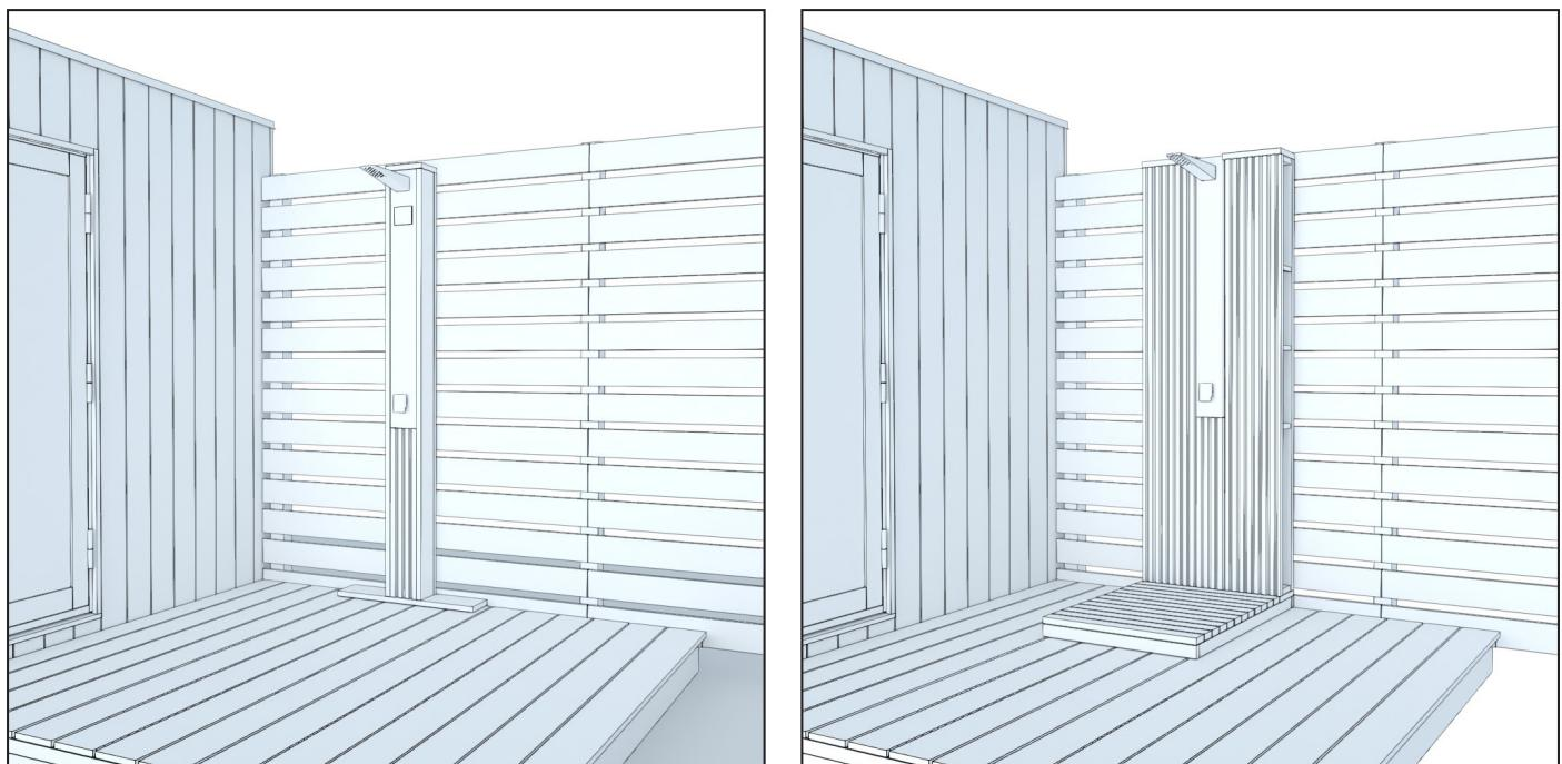
The Kirami FinVision® -outdoor shower (off terrace model) and Pillar models can be installed on any flat surface, such as an outdoor or rooftop terrace, near a hot tub, swimming pool, or sauna.
