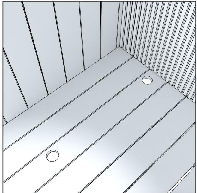
When Kirami FinVision® -outdoor shower Misty is ordered afterwards, holes must be drilled in the terrace module for the water inlet and outlet. The diameter of the hole to be drilled in the terrace is at least 73 mm.
