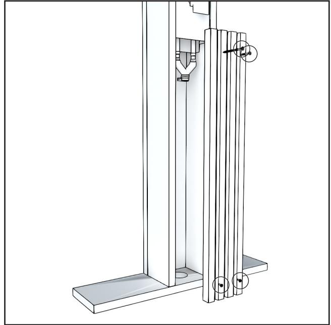
1. The inlet water connectors are located beneath the front panels. Remove the panels.
