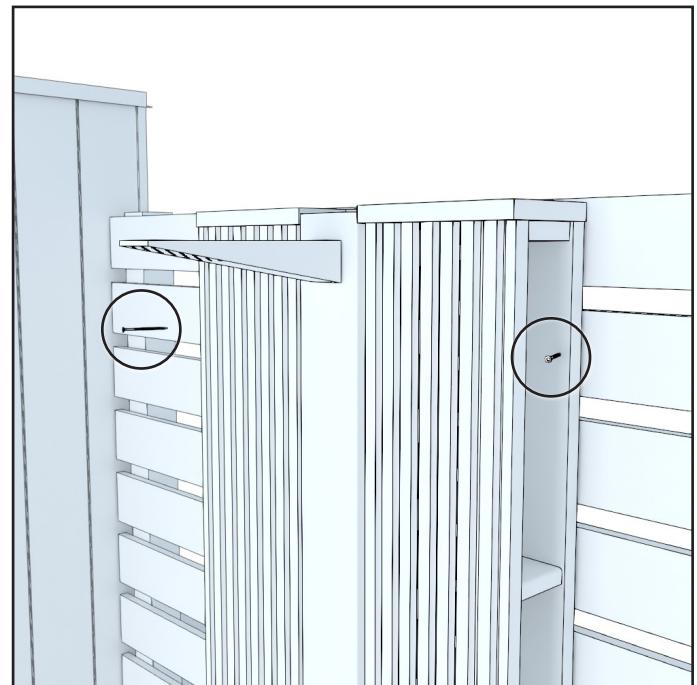
For an outdoor shower with a wall, first secure the base to the underlying material with four screws. Then, attach the top of the wall to the opposing material on both sides with screws.
