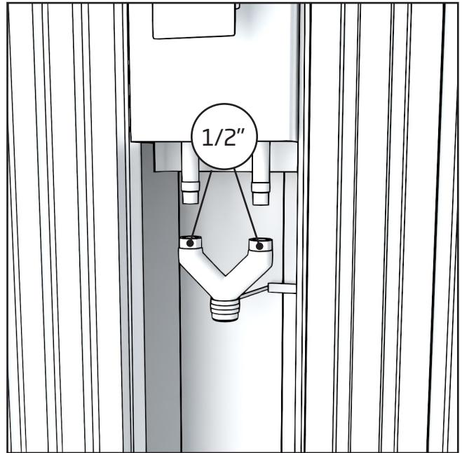
1. Remove the brass pipe splitter by turning the nuts counterclockwise and detaching the bracket from the wall.
