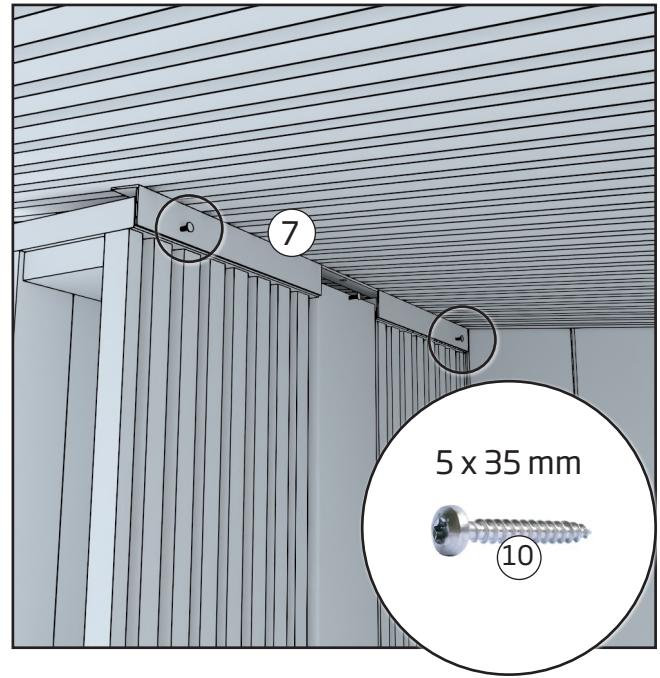
Position the outdoor shower against the connection plate and the back wall of the terrace. Attach the connection plate to the outdoor shower with screws.
