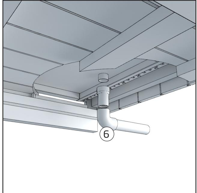
The base has a pre-made 50 mm drainage outlet for wastewater. When installing the Kirami FinVision® terrace, connect the pipe parts in the order shown in the image to route the outdoor shower drainage to the back of the module.
