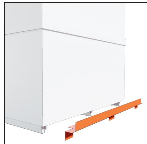
8. Remove the sheet metal from the rear bottom of the module. The sheet metal is attached with six screws
